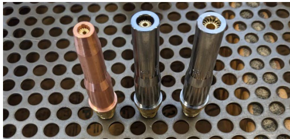
Figure 6. A variety of cutting tips (4", 8", 18" respectively).
