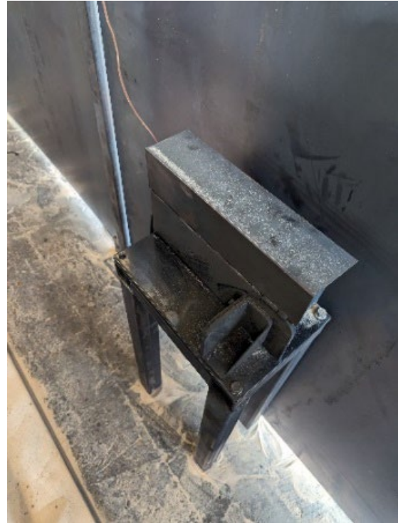
Figure 9. Igniter station for torch lighting.
