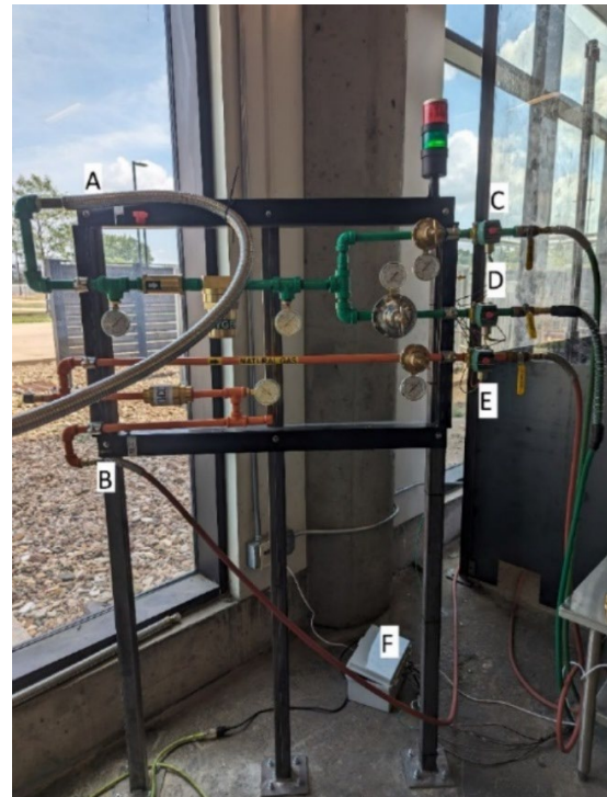
Figure 7. The oxygen and fuel manifold delivery system.
